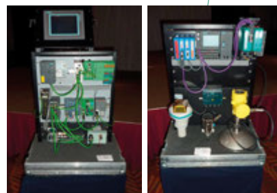
Multivendor demo with wireless integration of Profibus into a Profinet System.
