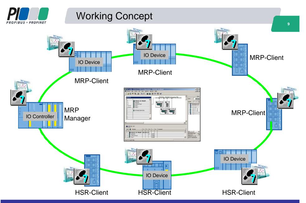
Every Device in the Ring needs to have configured ports for the ring
