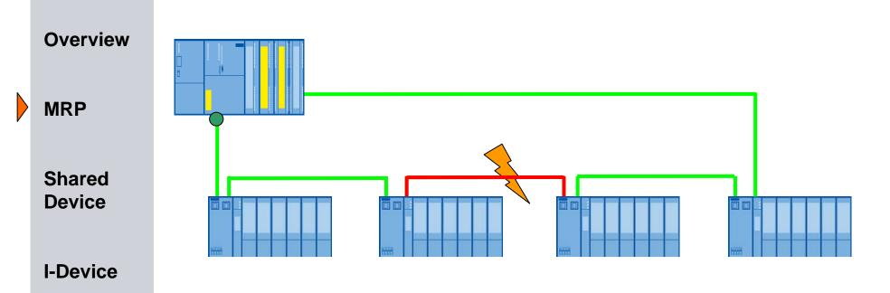
Web on Controller Most of PROFINET Devices are equipped with a built in Switch on Board! Line Structure is possible!
