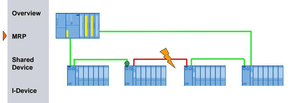
Web on Controller Most of PROFINET Devices are equipped with a built in Switch on Board! Line Structure is possible!
